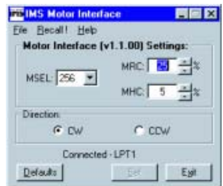
The IMS Motor Interface GUI simplifies MDrive configuring with a single screen interface.
